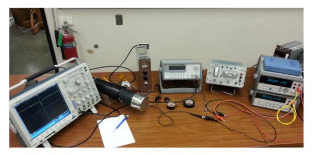
Begin with a contest to see how few photons you can count with your eye. There is an identical Sylvania 7377 light bulb set up at the end of a black tube. Hook this to your
